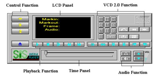
After installed the MPEGII Video Playback, you have created a **SiS MPEGII** program group which contains one icon --- SiS MMPlayer. Currently, SiS MMPlayer does not implement audio (most of the audio function buttons support only VGA 6225). Therefore, please turn off the **rate control** in the Configure (located in the Menu button). Follow the steps below, you will find this application not just easier to use but also more functional.
